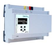
The device combines the central functions of a KNX bus line: Bus power supply with bus choke, KNX IP router and KNX IP interface with low space requirement. Comprehensive diagnostic functions. The KNX IP router in the LineMaster enables the forwarding of telegrams between different lines via a LAN (IP) as a fast backbone. The device also serves as a programming interface between a PC and the KNX bus (e.g. for the ETS®).
